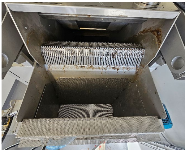
Photo 3 Collection basket for debris, 2 mm hole perforations.
